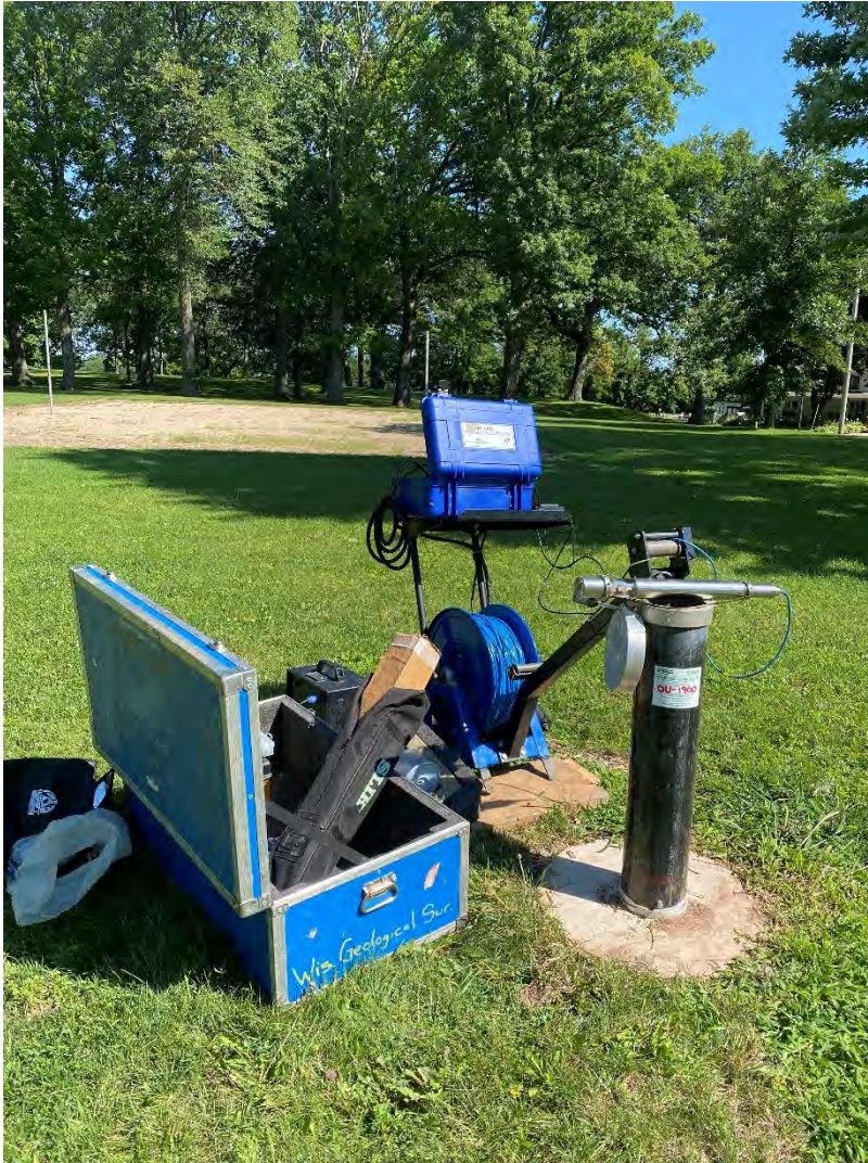
Figure 61. WGNHS video logging equipment set up to collect a borehole video from OU-1900 on August 10, 2022.
