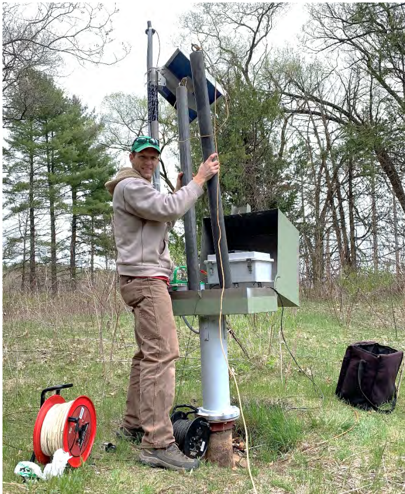
Figure 21. USGS-UMWSC staff performing a slug test on well DN-83. Staff member is holding two solid PVC slugs prior to dropping them inside the open well casing located out of view and inside the flip-top wells shelter. Image courtesy of U.S. Geological Survey.
