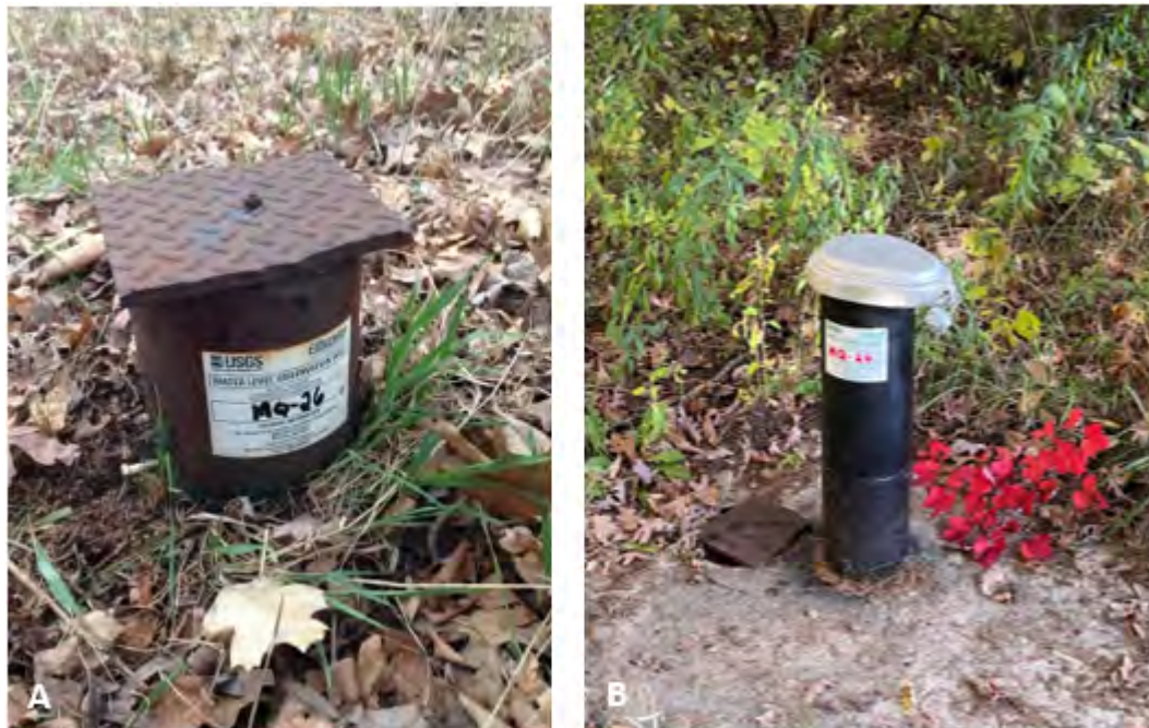
Figure 53. Well MQ-26. Panel A, old well head with square, steel cover plate, photo courtesy of U.S. Geological Survey. Panel B, new well head with extended protective cover pipe and locking cap installed May 26, 2022.
