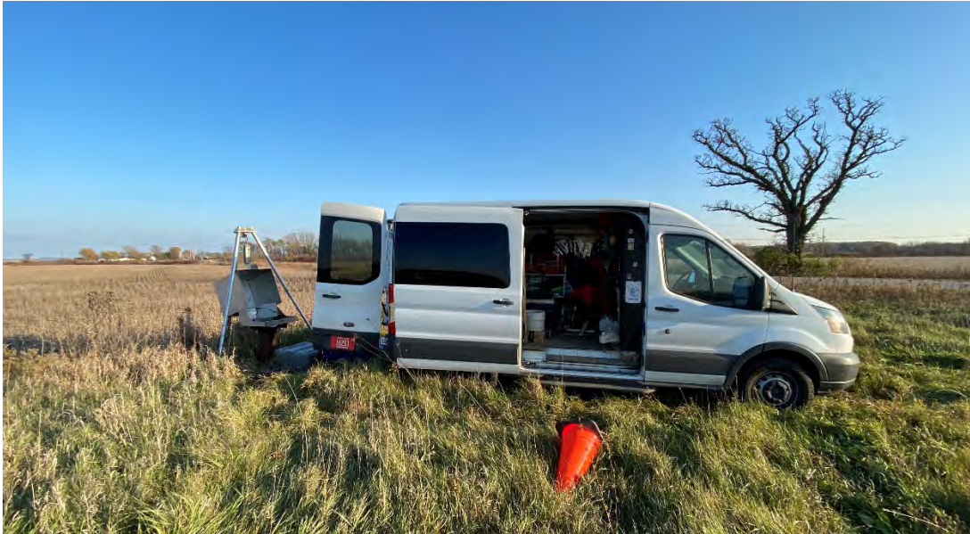
Figure 41. WGNHS geophysical logging van parked next to well FL-659 in preparation to collect down-hole geophysical logs. The tripod, which suspends the geophysical logging tools, can be seen set up over the well behind the van.
