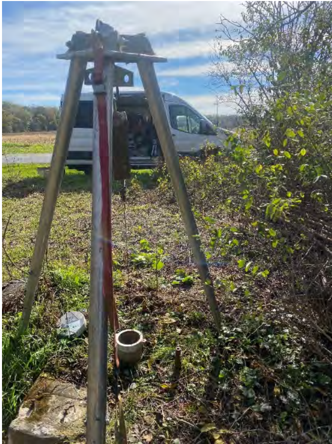
Figure 83. WGNHS collecting geophysical logs at well WW-09. Tripod is set up over well head, lowering the geophysical logging equipment into the well.
