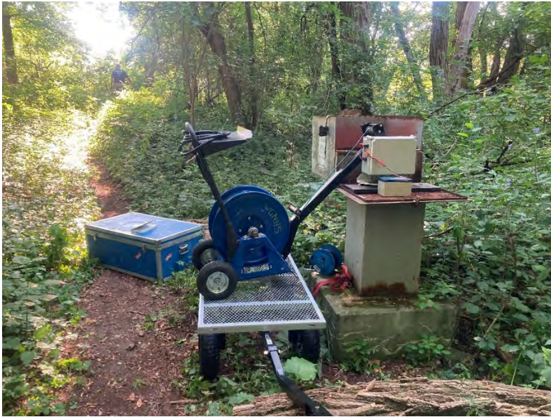
Figure 15. WGNHS setting up to collect a borehole video for well DN-64 on August 3, 2021. The video camera cable winch is shown set up on a wagon next to the well. The extended cable pulley suspended over the open well casing will lower the borehole video camera down the well. Inside the well shelter, the groundwater level float recorder is visible in the foreground (white box), blocking the view of the well opening.
