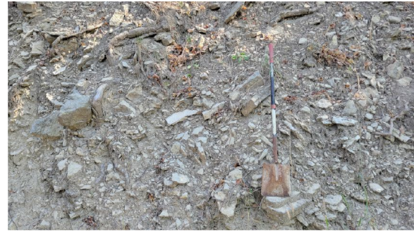
Figure 18. Example of coarse colluvium, map unit cc , showing angular and subangular boulders in a matrix of silt.
