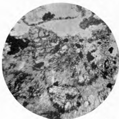
A. Oolites of siderite in chert. Without analyzer \times 40 . B. Same with analyzer. Shows coarse quartz in interstices.
