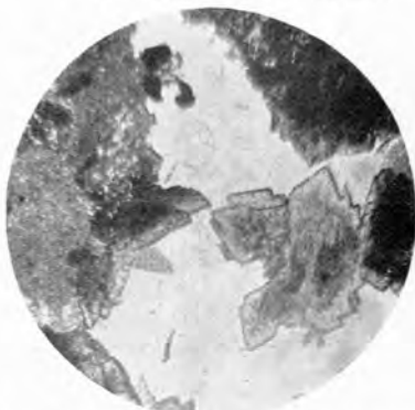
C. Oolitic chert. Without analyzer \times 40 . Shows coarse quartz in interstices. D. Same with analyzer. Note dense chert around rhombs of secondary carbonate.
