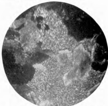
C. Oolitic chert. Without analyzer \times 40 . Shows coarse quartz in interstices. D. Same with analyzer. Note dense chert around rhombs of secondary carbonate.
