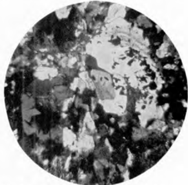
A. Oolitic chert. Without analyzer \times 40 . Carbonate replaced by quartz and magnetite. B. Same, with analyzer.
